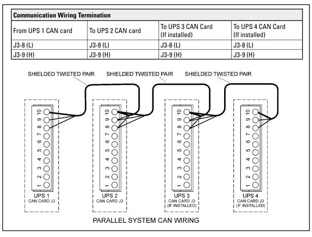
Figure 23 Communication cabling wiring
